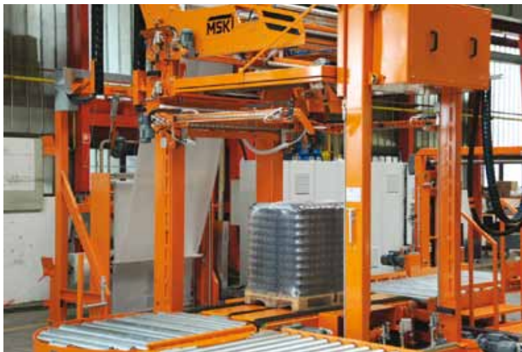
Secure shrinkwrapping of glass pallets with border-free packaging due to the contact-free film hooding of the MSK Multitech 2010 shrinkwrapping machine.
