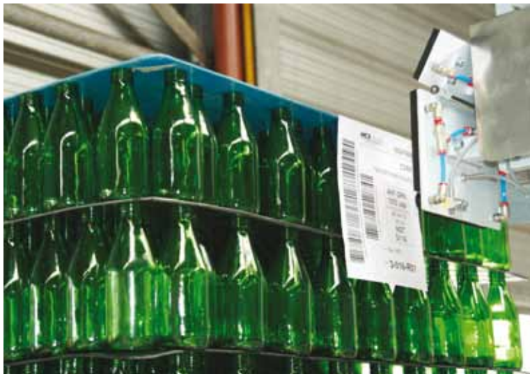
The MSK labelling system enables good readability at the side of the pallet by use of plastic trays.
