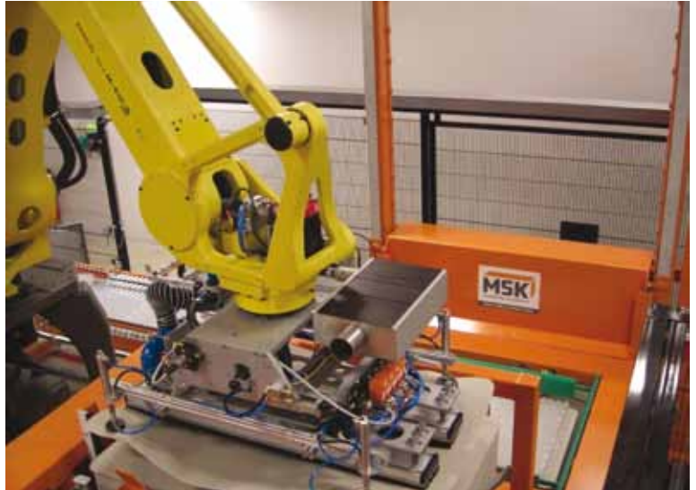
THE ROBOT ALSO HANDLES THE APPLICATION OF INTERLAYERS
