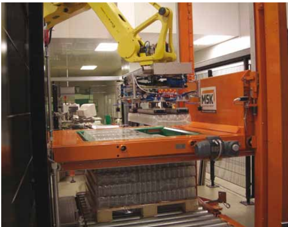
ROBOT PALLETISING OF CLEAN PACKS AT SGD KIPFENBERG GMBH
